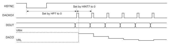
The internally generated digital data DOUT is input to the internal D/A converter, latched by the D/A converter clock input from DACKI, and output from DACO2, 1 and 0 as an analog signal.
